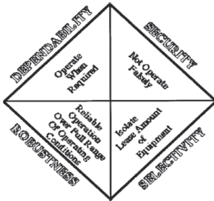
FIGURE 6.1 Protection and control system characteristics.
